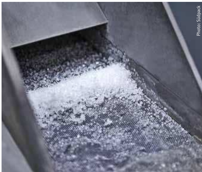
The starting material for Südpack's compounds is its own clean film scraps.
