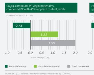
Reduction of the carbon footprint with processing of recyclates
